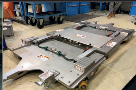
This is detail pic of the ACMT = Advanced Column Moving Trolley to lift and move Columns up to 20 tons. Height above floor is 170mm, can adjust by telescoping rails to 3 different column sizes and lifting/lowering of Hydraulic cylinders is by remote-control.
