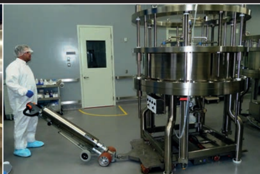
PowerAttack and a purpose-designed trolley to lift and transport „columns“ for the BioTech industry
